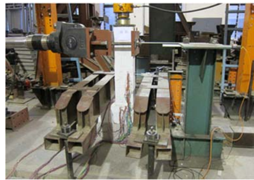
图2 型钢再生混凝土柱低周反复荷载试验 Fig. 2 Cyclic loading tests of steel reinforced recycled concrete(SRRC) columns
