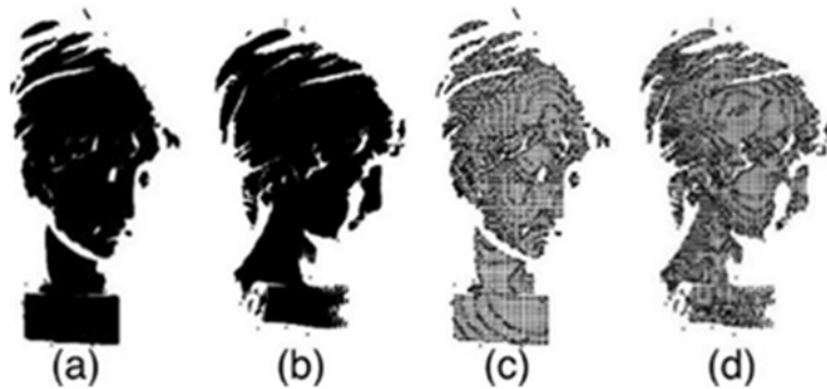
图9 点云和降采样点云。(a-b)点云 P 和 Q ; (c-d)降采样后的点云 \bar{P} 和 \bar{Q} Fig. 9 Point clouds and down sampled point clouds. (a-b) Point cloud P and Q ; (c-d) down sampled point clouds \bar{P} and \bar{Q}
