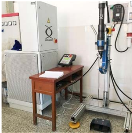
图1 Böllhoff 自冲铆接设备 Fig. 1 Self-piercing riveting (SPR) equipment of Böllhoff
