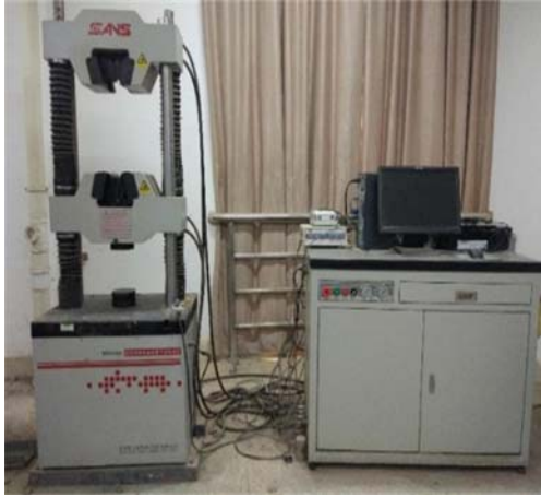
图 3 SHT4305 型微机控制电液伺服万能试验机 Fig. 3 SHT4305 microcomputer control electro-hydraulic servo universal testing machine
