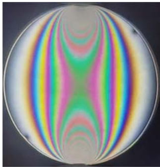
图 1 竖向对径荷载下光弹模型彩色条纹图 Fig.1 Color stripe diagram of the photoelastic model under vertical opposite radial load
