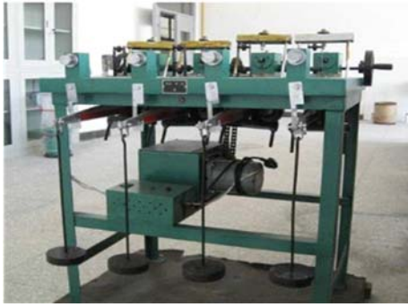
图 16 DSJ-2 电动四联等应变直剪仪 Fig. 16 DSJ-2 Electric quadruple strain straight shear instrument
