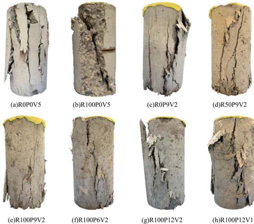
图3 典型试件破坏形态图 Fig.3 Typical failure pattern of specimens
