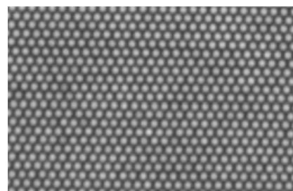
图 7 空白背景下传像束成像的蜂窝伪影 Fig. 7 Honeycomb artifacts in image beam imaging on a blank background
